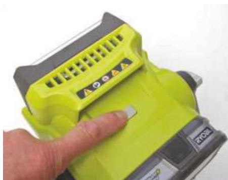
A single push button activates the light
